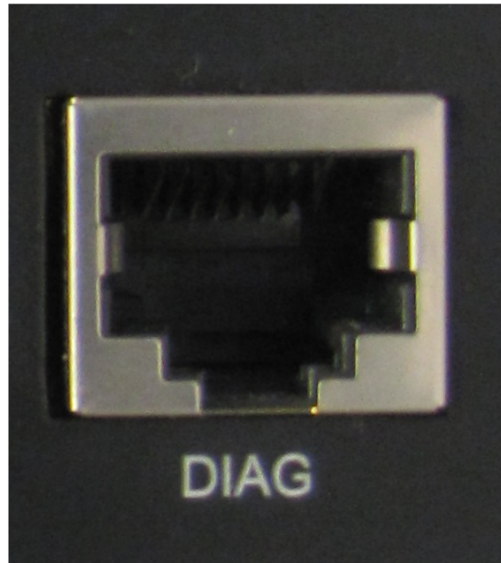
Figure 5 FSM104/FSM204 Diag port on front panel
