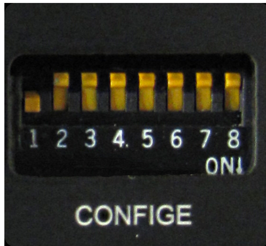
Figure 4 FSM104/FSM204 DIP Switches on front panel
