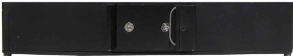
Figure 16 Installing DIN RAIL mounting clamp on FSM203 Desktop (Right or Left side)
