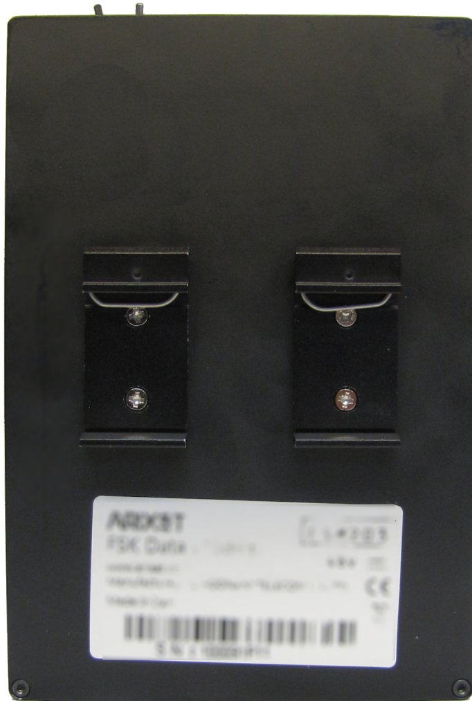
Figure 17 Installing double DIN RAIL mounting clamps on FSM203 Desktop (Back side)
